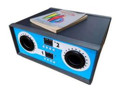
The BL672 is a benchtop blackbody calibration source utilizing a digital indicating temperature ambient 30°C to 50°C (86F to 122F). Two 60mm diameter end closed tube is heated or cooled with an internal solid state thermoelectric heat pump. It has a built-in digital temperature controller to provide accurate, stable temperature as well as to provide readout.
