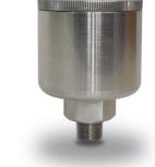
The *Track-It*<sup>™</sup> Pressure/Temperature Vacuum/ Temperature Data Logger can be ordered in several pressure or vacuum ranges: 0-3, 0-35, 0-150, 0-350, 0-550, 0-2000, 0-5800, 0-8700 and 0-14500 PSI or 760-380 and 760-0 Torr. The logger is packaged in a rugged submersible 316L stainless steel housing and has a standard 1/4" NPT fitting (1/2" NPT for 8700 and 14,500 ranges). The replaceable battery has up to a 5 year life.
