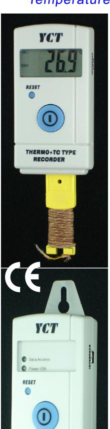
THERMO+TC TYPE RECORDER The Datalogger is a miniature, battery powered, stand alone, thermocouple based temperature recorder, This is an all-in-one compact, portable, easy to use device that will measure and record up to 10,000 measurements per channel. The storage medium is non-volatile solid state memory, providing maximum data security even if the battery becomes discharged.
