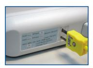
Built-in jack supports any K-type TC probe with "mini"-style connector
