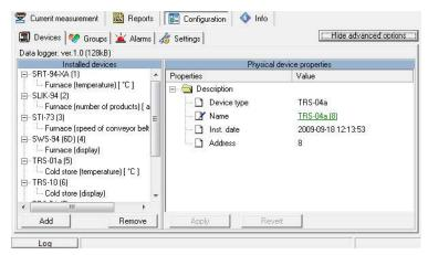
SimCorder is designed for acquisition, archiving, visualization and reporting of measurement data from SIMEX products equipped with RS-485 serial communication interface with Modbus RTU protocol. Converters like RS-485/USB or RS-485/RS-232 allow connecting multiple devices to a computer via USB or RS-232 port. Both devices can be found in SIMEX product range.
