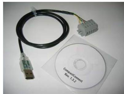
Fig. 3.5: USB programming adaptor incl. terminal block and software CD [TM-USBK-CS]
