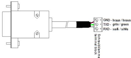
**Fig. 10.3: Correct wiring**
