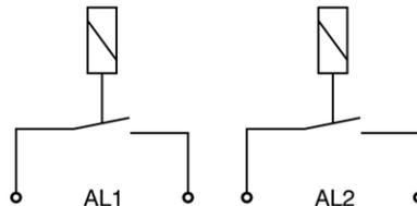
**Fig. 10.6: Relays-Interface with pin assignment**
