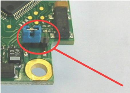
**Fig. 9.4: Connector (Jumper)**
