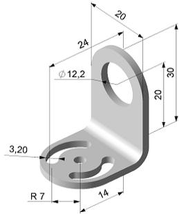
**Fig. 8.5: Mounting bracket [TM-FB-CT]**
