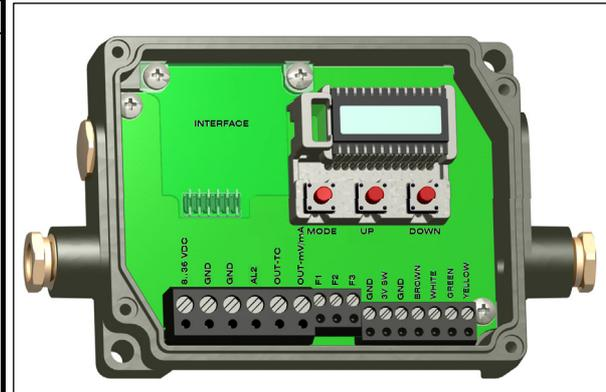
**Abb. 9.2: Opened controller with terminal connections**
