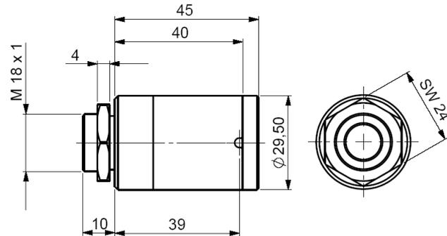
Fig. 8.2 Massive housing (Standard on CTH)
