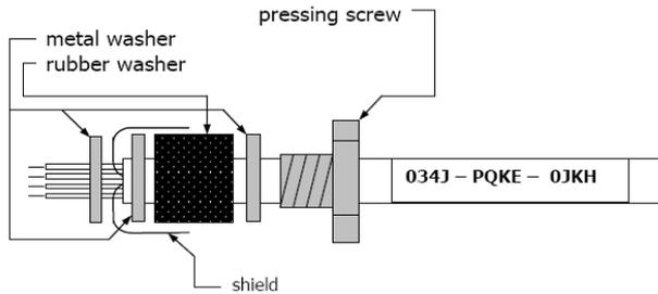
**Fig. 9.3: Cable Assembling**
