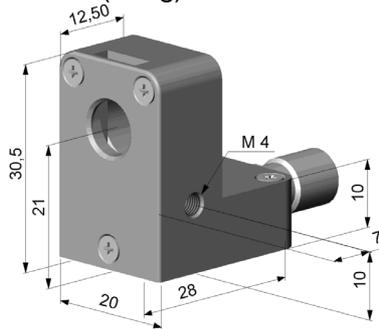
Fig. 8.11: Laminar air purge collar [TM-APL-CT]
