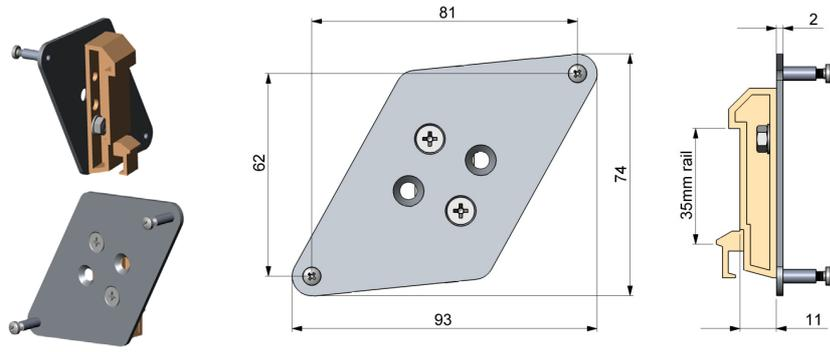
**Fig. 8.14: Rail mount adapter for controller [TM-TRAIL-CT]**
