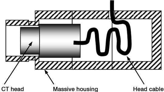
Fig. 8.17: Massive housing
