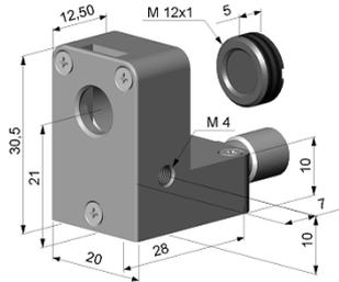
**Fig. 7.2: Laminar air purge with integrated CF lens [TM-APLCF-CT]**
