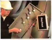
... attach Thermocouples to product or test piece.
