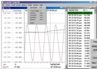
The real power of the COMPANION software is when it is used in conjunction with a serial communications link with the Datagraph recorder. Users can monitor, configure and control up to 31 recorders with the RS485 MODBUS option or control remote locations via a MODEM link to the recorder RS-232 interface. Whatever the application, the COMPANION software puts you in complete control.
