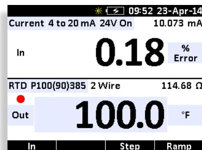
Online % error calculation, fast and responsive reading, for calibration and adjustment tasks
