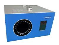
With isothermal cavity, the BL672S is a portable blackbody calibration source utilizing a digital indicating temperature ambient 20°C to 50°C (68F to 122F). The 80 mm diameter end closed tube is heated or cooled with an internal solid state thermoelectric heat pump. It has a built-in digital temperature controller to provide accurate, stable temperature as well as to provide readout.
