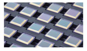
E2n/E3n -17µm detector
