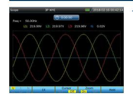
View the voltage/current waveform and readings.
