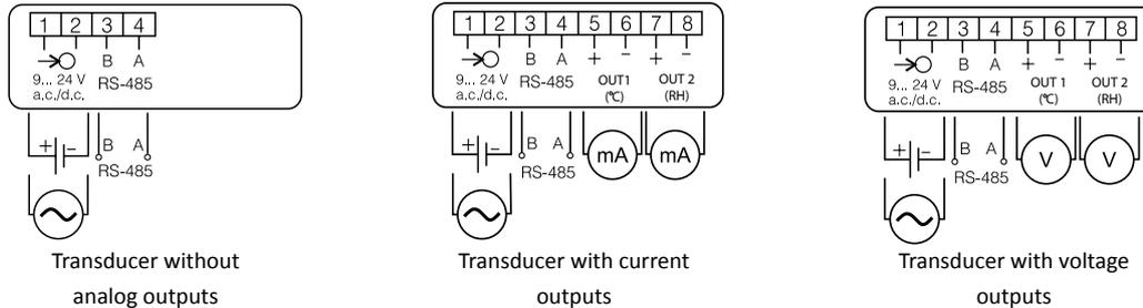
**Fig. 1** Connection way of electric signals – P18, P18D.
