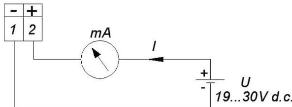
**Fig. 2** Connection way of electric signals – P18L
