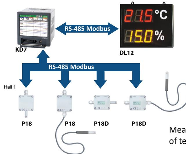
Measurement and recording of temperature and humidity.
