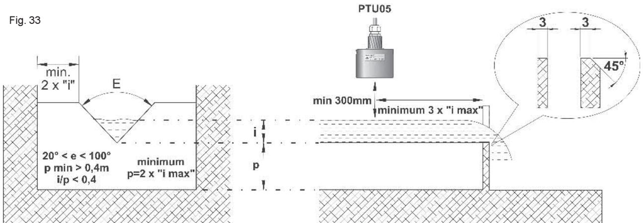
To parity of flow, the triangular weir has a loss of load inversely proportional to the opening angle "E"
