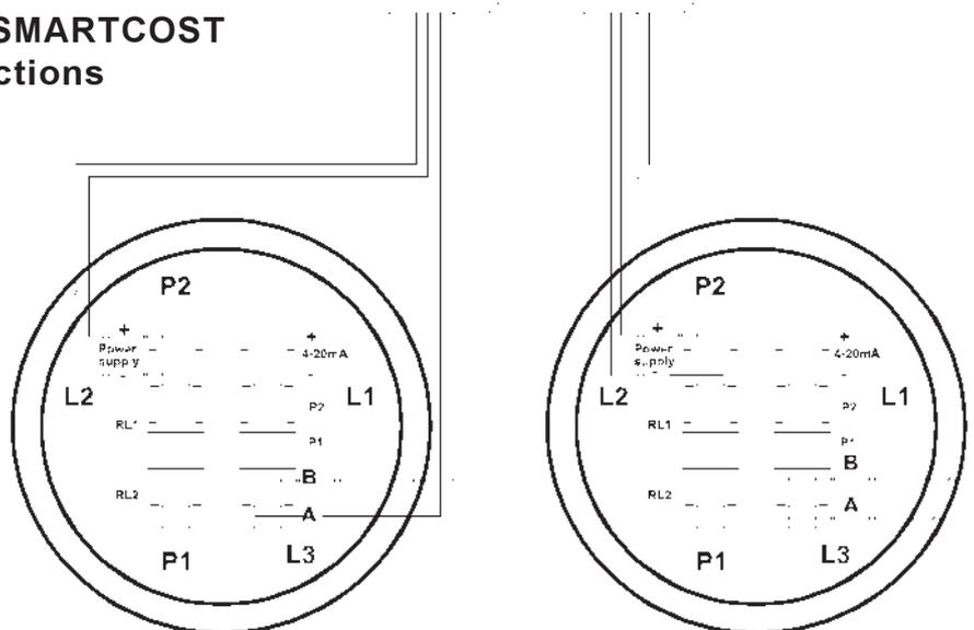
**Warning.** For dual channel configuration, it is necessary set the internal Unit Identification Device (UID) by the RS485 ports. To program different UID codes for each SmartCost transmitter needs to connect the CH1 SmartCost disconnecting the CH2 SmartCost extracting connector then refer to the procedure in “Configuration/ProbeCH1-Selection”. Successively connect CH2 SmartCost, disconnecting the CH1 SmartCost and refer to “Configuration/ ProbeCH2-Selection” (see 1.3.1 and 1.4.1).
