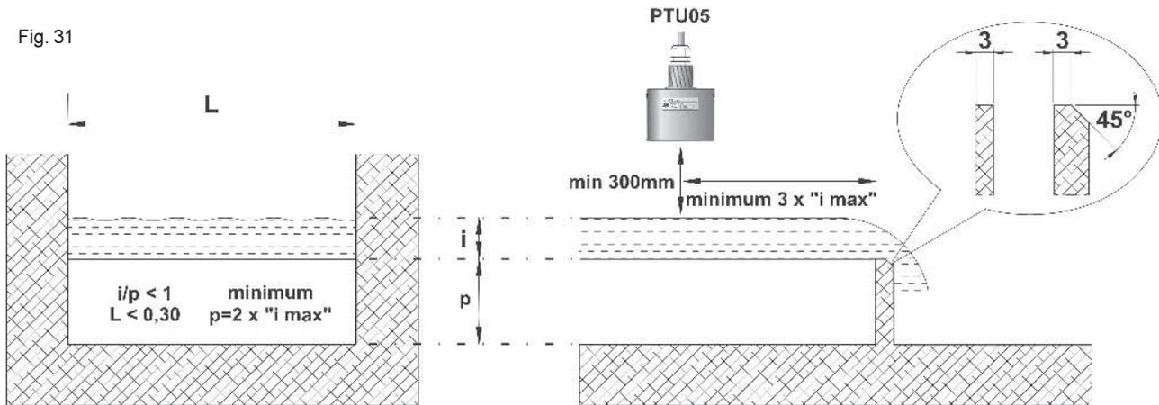
To parity of flow, the "Bazin" weir is what has a smallest loss of load, it that is requires a smallest level height "i"
