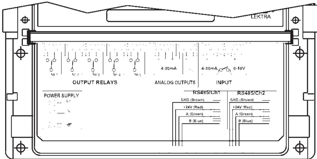
**FIG. 10 - Dual channel PTU electrical connections**
