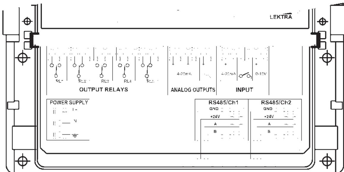
**Fig.11 - Dual channel SMARTCOST electrical connections**
