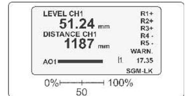
Fig. 20 - Display example: has stayed selected first "DISTANCE CH1," then "LEVEL CH1"
