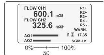
Fig. 28 - Display example: has stayed selected first "FLOW CH2," then "FLOW CH1"
