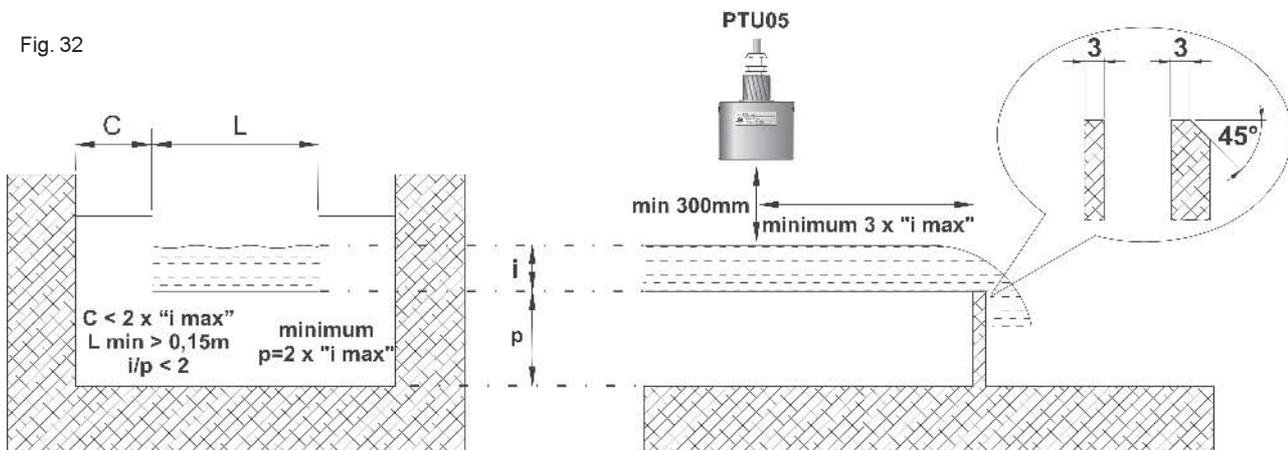
The "Francis" weir comes generally used when is required a better accuracy than the "Bazin" weir, but it present a bigger loss of load.
