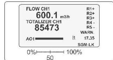
Fig. 27 - Display example: has stayed selected first "TOTALIZER CH1," then "FLOW CH1"
