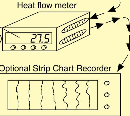
Records Rate in BTU/Ft<sup>2</sup>Hr or Watts/Meter<sup>2</sup>
