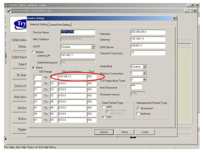
Step3.Run DSM set up *TRP-C37M as Server* and be sure the IP and port as same as client setting.
