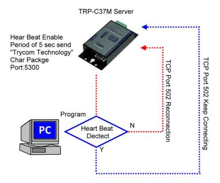
Step1: Run TRP-C37X DSM utility to set up the heart beat enable.
