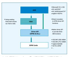
work with your applications in both ways. Its GPIB-32.DLL provides binary compatibility with the popular NI-488.2\* driver software. The USB-3488A and LPCI-3488A also provide VISA library support that can be used with most common instrument drivers written by instrument vendors. Regardless if you are using VC++, VB, Delphi, LabVIEW $^{\text{TM}}$ \*, or any other T&M ADE, ADLINK GPIB interface cards are the most cost-effective GPIB solutions compatible with all your applications.
