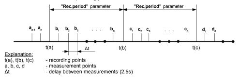
Fig. 6.2. Principle of measurement recording
