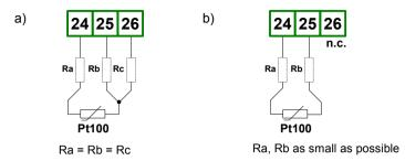
Fig. 4.9. Connection of Pt100 sensors for channel no 1: a) 3-wires circuit; b) 2-wires circuit;
