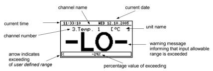
Fig. 6.10. Exceeding allowable range in "Single channel" mode
