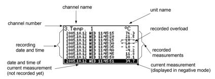
Fig. 6.11. Unit in "Measurements list" measurement results presentation mode.
