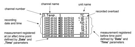
Fig. 6.12. Unit in "Measurements list" measurement results presentation mode. "List type" parameter set as "historic".
