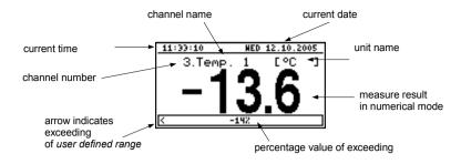
Fig. 6.9. Exceeding user defined range in "Single channel" mode
