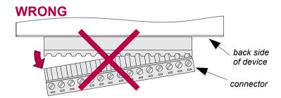
Fig. 4.3. Connectors removing method
