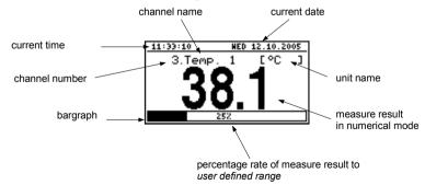
Fig. 6.8. Unit in "Single channel" result presentation mode
