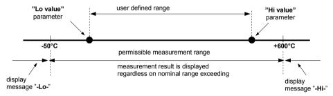
Fig. 6.1. Definition of measurement ranges
