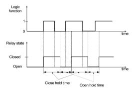
Fig. 6.26. Working relay diagram in "N.O." mode. "Open hold time" and "Closed hold time" greater than 0, "Open delay" and "Close delay" equals 0.
