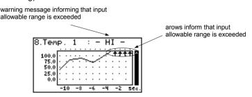
Fig. 6.15. Exceeding the upper limit of the allowable measurement range
