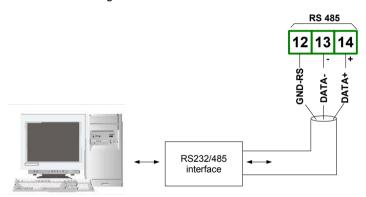
Fig. 4.10. Connection of RS-485 transmission signals
