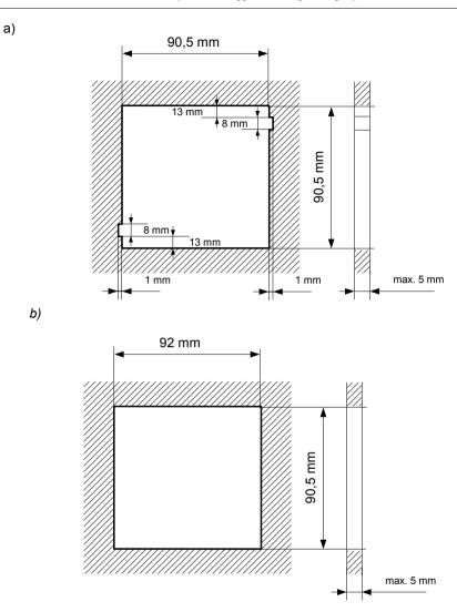
Fig. 4.1. Mounting hole dimensions: a) recommended b) allowable
