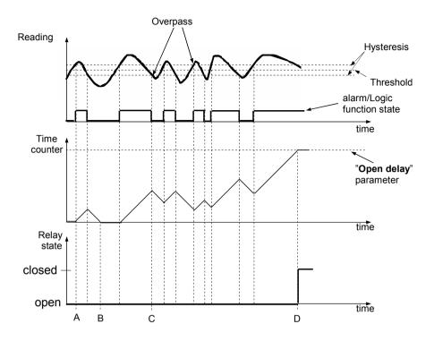
Fig. 6.27. Working output controlled by single channel alarm with large reading oscillations.
