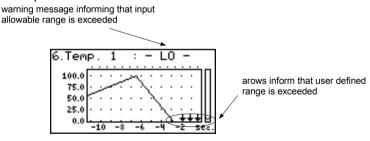
Fig. 6.16. Exceeding lower limit of the allowable measurement range
