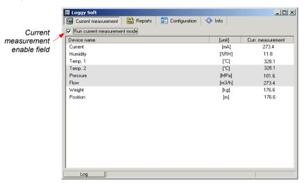
Fig. 3.2. Current measurement menu
