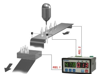
A basic advantage of the **SLN-94** counters is an exceptionally easy setting change. The changing is performed by 3 buttons located under each decade of the SV threshold value display (green). The current value can be read on the PV display (red). Consequently, the counter operator is able to change the settings quickly and easily. The counting can be performed up-down or down-up, and the control is by means of the relay output.
