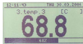
the current value in the selected channel The height of the digits: 18 mm
