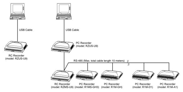
Non-isolated between USB and RS-485. RS-485 cable length is limited within 10 meters.
