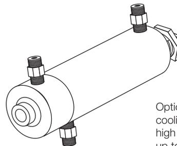
Optional water/air cooling/purging system for high temperature environments up to 260°C (500°F)
